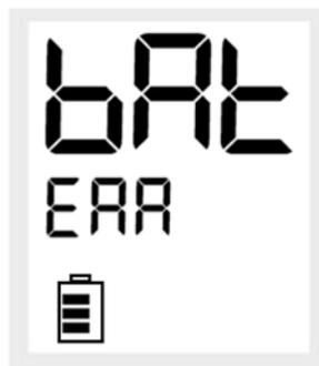
The battery may not successfully charge for a number of reasons: the battery may be overcharged, the battery may not be taking a charge in a reasonable amount of time, the battery may be too warm to be charged without causing damage to its internal cells, or the battery charger may have an internal fault.
