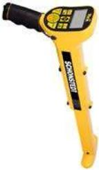
In the passive mode, the transmitter is not used at all. Instead, the receiver searches for an appropriate harmonic of 60 or 50 Hz signals (factory preset). These signals are typically present in energized power cables, making it possible to locate them without using a transmitter to impose a tracing signal onto them.
