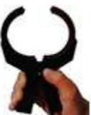
In the inductive clamp mode, the transmitter imposes a signal of the selected frequency onto the pipe or cable to be traced. It does so by energizing a clamp that is placed so that it is completely encircling the pipe or cable at a point where the pipe/cable comes up to the surface of the ground (a
